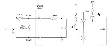
High Speed Counter Circuit – Negative Logic Connection
