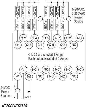
Wiring Diagram, IC200UER016
