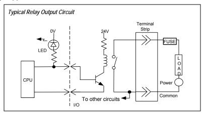
Installing suitable suppression across inductive loads enhances reliability of relay contacts. When switching inductive loads, relay contact life approaches resistive load contact life if suppression circuits are used. The 1A, 100V diode shown in the typical DC load suppression circuit is an industry standard 1N4934.
