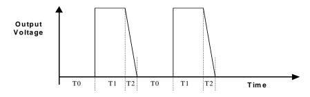
Pulse Train Outputs can be used to control stepper motors.
