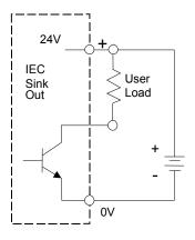
Typical High-Speed Counter Connections
