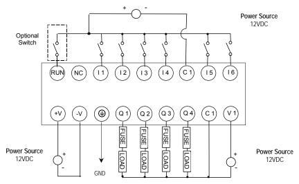
VersaMax Nano PLC IC200NDD101 has six 24VDC inputs and four DC transistor outputs. It uses +24VDC nominal input power for PLC operation.
