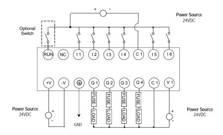
VersaMax Nano PLC IC200NDR001 has six 24VDC inputs, and four normallyopen 2 Amp relay outputs that can control 5 to 30VDC or 5 to 250VAC output devices. It uses +12VDC nominal input power for PLC operation.
