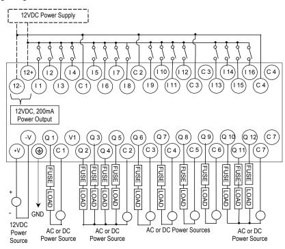
IC200UDR010 28 Point Micro PLC, (16) 24VDC In, (1) 24VDC Out, (11) Relay Out, 24VDC PS IC200UDR228 28 Point Micro PLC, (16) 24 VC In, (1) 24VDC Out, (11) Relay Out, 12/24 VDC PS
