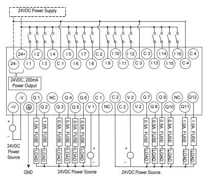
The maximum current that can be used for output points Q1, Q2, Q11 and Q12 is lower for ambient temperatures above 50 degrees C
