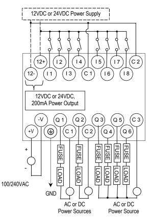
VersaMax Micro PLC IC200UDR002 accepts eight DC inputs and provides six normally-open 2 Amp relay outputs that can control 5 to 30 VDC or 5 to 250VAC output devices. It uses +24VDC nominal input power for PLC operation.
