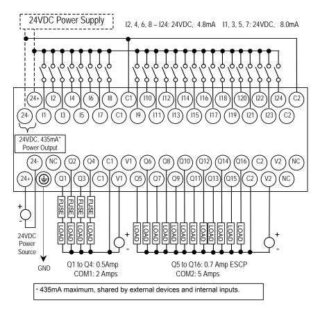
VersaMax Micro PLC IC200UDD240 accepts twenty-four DC inputs and provides sixteen DC outputs. It uses +24VDC nominal input power for PLC operation.
