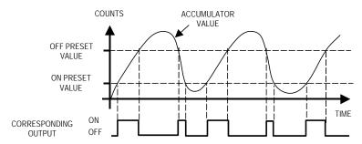
If the output is enabled for the High-speed Counter being used, the output turns on as described in the Type A and Type B counter sections.
