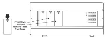
2. If a port-type Option Module is being installed, orient the connector on the Option Module with the connector in the Micro PLC. Be careful to avoid contact with the exposed components in the module.
