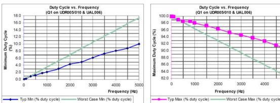
Duty Cycle Limits: with 1.5k ohm pulldown resistor - UDR005/006/010 & UAL004/005/006
