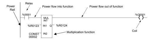
The flow of logical power through each rung is controlled by a set of simple program functions that work like mechanical relays and output coils. Whether or not a relay passes logical power flow along the rung depends on the content of a memory location with which the relay has been associated in the program. For instance, a relay might pass power flow if its associated memory location contained the value 1. The same relay would not pass power flow if the memory location contained the value 0.
