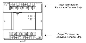
The terminal block assemblies of a Micro PLC can be removed to perform wiring. For example, a 14-point unit (shown above) has two removable terminal assemblies.
