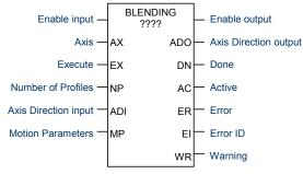
The channel's Output Enable bit (for example, Q0505 for channel 1) must be set to 1 to use this or any other motion function block. If the Output Enable bit is not 1, the function will not execute, and a Channel Enable error will be reported.
