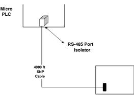
When installing the Port Isolator on a panel, you will need to provide two #6-32 mounting screws.
