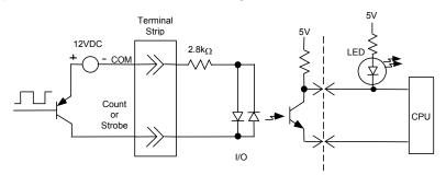
High Speed Counter Circuit – Negative Logic Connection
