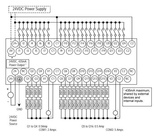
IC200UDR040 40 Point Micro PLC, (24) 24VDC In, (16) Relay Out, 24VDC Power Supply IC200UDR140 40 Point Micro PLC, (24) 24VDC In, (16) Relay Out, 120/240VAC Power Supply IC200UDR440 40 Point Micro PLC, (24) 24VDC In, (16) Relay Out, 12/24VDC Power Supply
