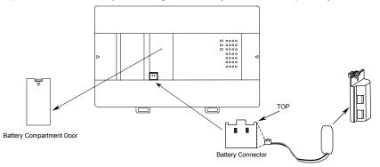
*For a cylinder-type battery*, tuck in the wires and snap the battery holder (see the illustration above) onto the VersaMax Micro PLC. The original battery compartment door is no longer needed.
