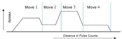
Because each Blend profile is equal to a normal ramping profile, a Pulse train with Ramp can be done using a Blended move with just one blending profile. Use this method if the hardware configuration selected is 4 Type A\_32 or 1 Type A/1 Type B\_32.
