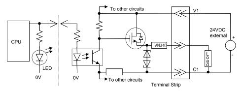
For Micro -10, -14, -23 and -28 PLCs, when using the outputs as PWM or Pulse Train Outputs, and for duty cycles in the lower ranges (5% and lower), a pulldown resistor must be connected between the output point (Q1-Q3) and the common terminal (C1). A 1.5 Kohm, 0.5 watt resistor is recommended.
