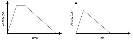
If the Ramp output is already decelerating (because the number of pulses has been reached) when the Enable Output bit transitions from 1 to 0, the Pulse Train output continues decelerating at the same rate.
