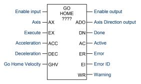
The channel's Output Enable bit (for example, Q0505 for channel 1) must be set to 1 to use this or any other motion function block. If the Output Enable bit is not 1, the function will not execute, and a Channel Enable error will be reported.
