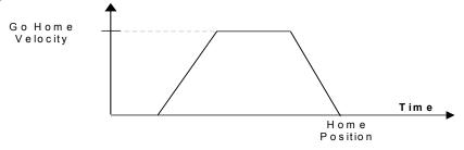
If a Home Offset was set up during execution of the Find Home function, the Go Home function causes the motor to move to the Home Offset position instead.
