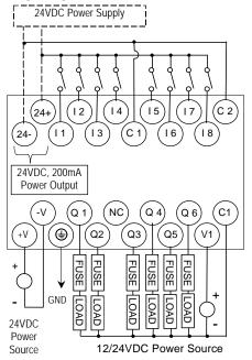
The maximum current that can be used for output points Q1 and Q2 is lower for ambient temperatures above 50 degrees C.
