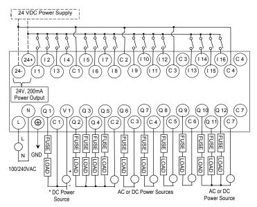
VersaMax Micro PLC IC200UDR006 accepts sixteen 12VDC inputs and provides twelve normally-open 2 Amp relay outputs. It uses +12VDC nominal input power.
