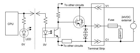
Typical Transistor Output Circuit 24 VDC
