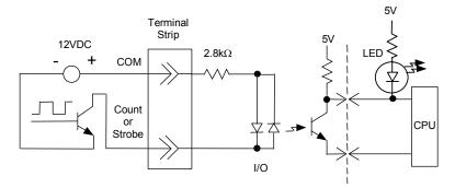
When I1-I6 on a Micro PLC are used as High-speed Counter inputs, the input switches should be solid state to prevent switch bouncing, which could cause unintended high speed counter counts or strobe input signals.
