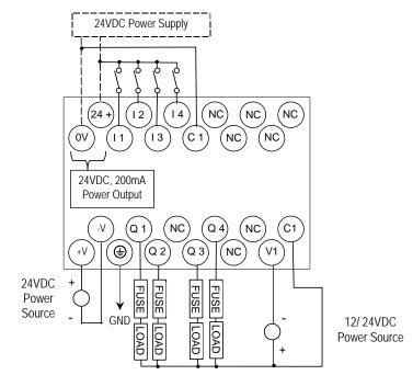
VersaMax Micro PLC Expansion Unit IC200UEC208 accepts four 24VDC inputs and provides four normally-open 2 Amp relay outputs that can control 5 to 30 VDC or 5 to 250VAC output devices. It requires +24VDC nominal input power.
