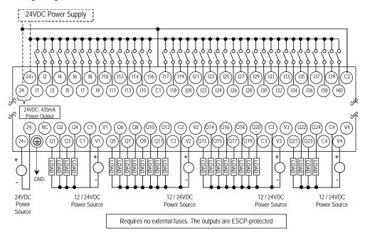
VersaMax Micro PLC IC200UDD164 accepts forty DC inputs and provides twentyfour DC outputs. It uses +24VDC nominal input power for PLC operation.
