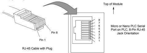
Note: There is no shield or frame-ground or shield pin on this connector.
