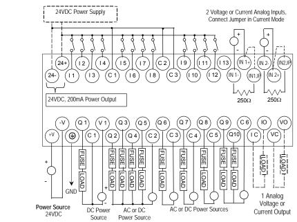
Wiring Diagram, IC200UAL005
