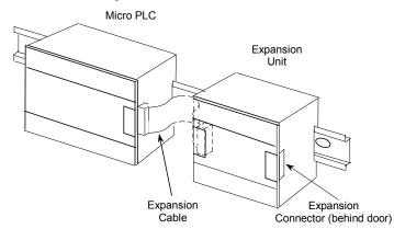
The Expansion Unit(s) and Micro PLC must be connected in the same orientation. Connecting an Expansion Unit "upside down" will damage the DC input circuit when the system is powered up.
