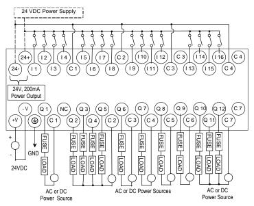
IC200UEX213 28 Point Micro PLC Expansion Unit, (16) 12VDC In, (12) Relay Out, 12VDC Power Supply
