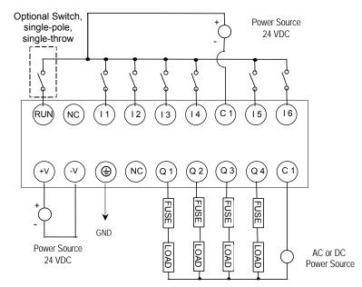
VersaMax Nano PLC IC200NDR010 has six 24VDC inputs, and four normallyopen 2 Amp relay outputs that can control 5 to 30VDC or 5 to 250VAC output devices. It uses +12VDC nominal input power for PLC operation.
