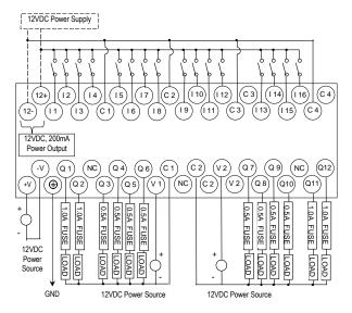
IC200UEX222 28 Point Micro PLC Expansion Unit, (16) 24VDC In, (12) 24VDC Out with ESCP, 24VDC Power Supply
