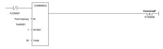
The following rung sets the bit Commreq Complete (%T7), which keeps the COMMREQ from being issued more than once and keeps the status from being overwritten.
