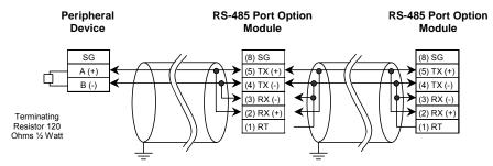
Connections: Peripheral Device to RS-485 Option Module
