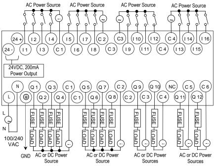
Outputs Q 1 - Q 10 are rated at 2.0 Amps each. Outputs Q 11 and Q 12 are rated at 10.0 Amps each.
