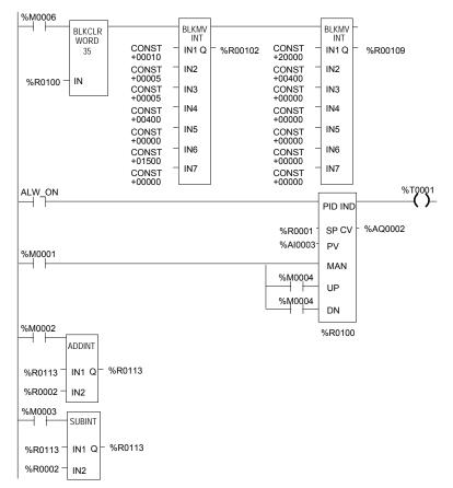
The block can be switched to Manual mode with %M1 so that the Manual Command, %R113, can be adjusted. Bits %M4 or %M5 can be used to increase or decrease %R113 and the PID CV and integrator by 1 every 100 MSec solution. For faster manual operation, bits %M2 and %M3 can be used to add or subtract the value in %R2 to/from %R113 every PLC sweep. The %T1 output is on when the PID is OK.
